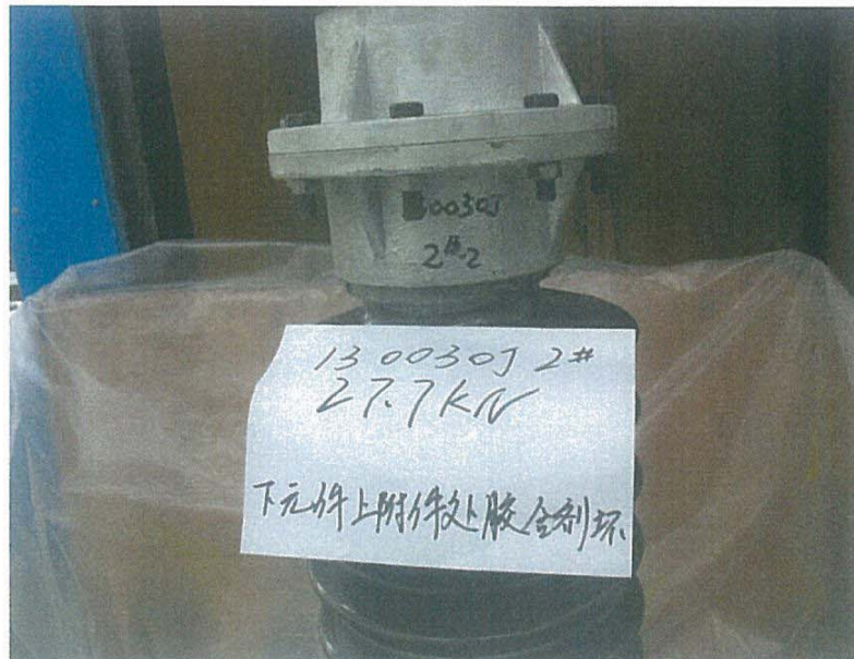
2号样品破坏部位/failure spot of No.2 sample
